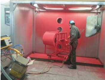
Power Recovery Booth Painting Booth
