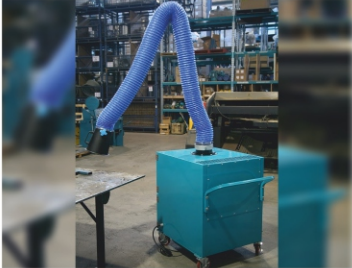
Fume Extraction System
